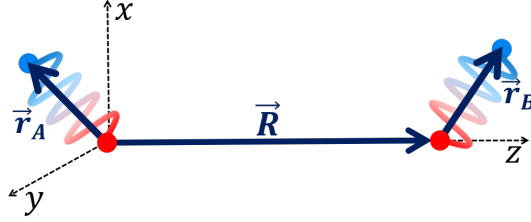
Figure 2.2: Two interacting dipole oscillators A and B separated by a distance R on the z -axis.
